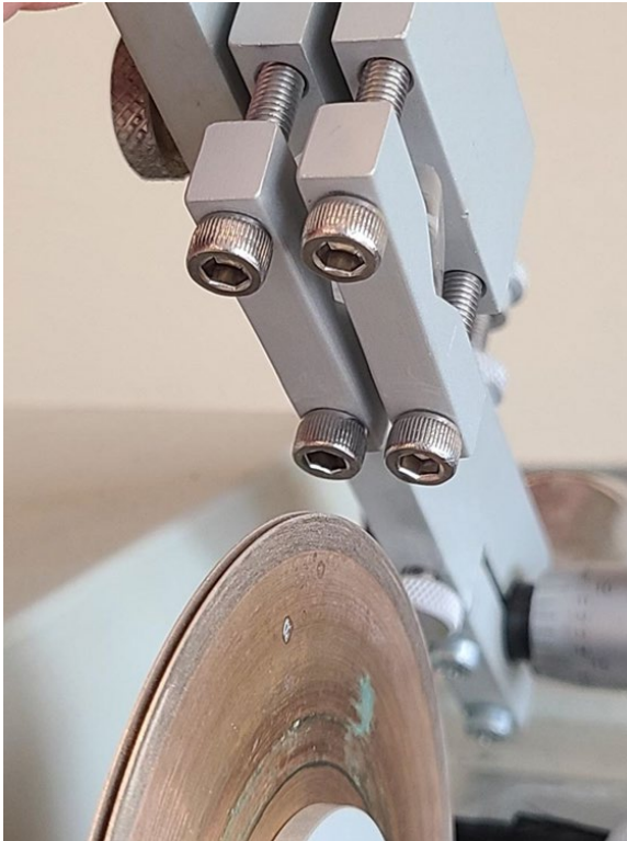
Figure D 2 - Thin-sectioning set up for otoliths mounted within epoxy blocks.
